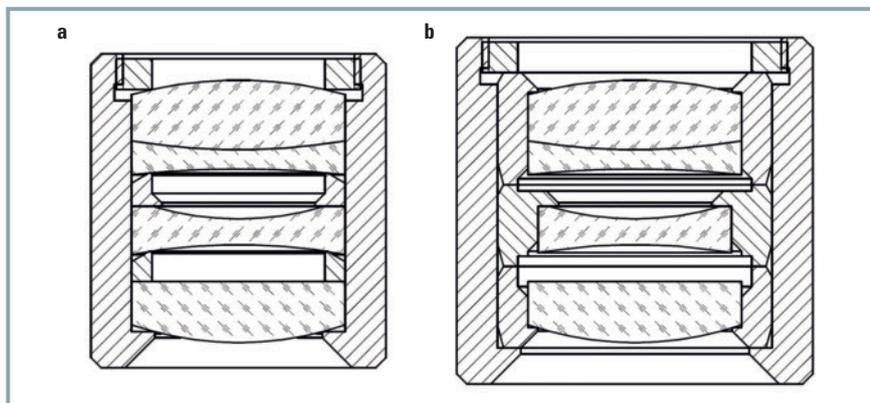
5 Mounting examples with (a) classical drop-in assemblies and (b) precision mounting technologies with sub-mounted optical components
