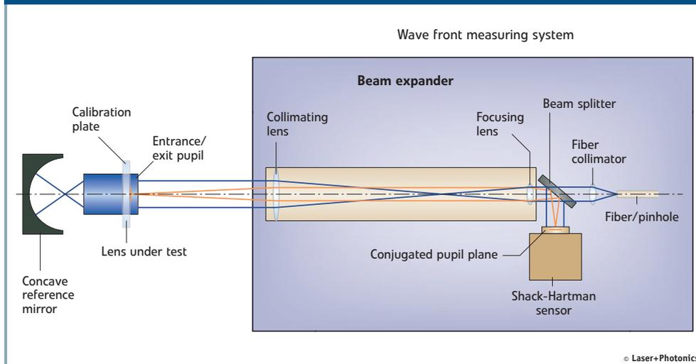
6 Diagram of the wavefront measuring system implemented by Linos for measuring high-resolution lenses for UV applications
