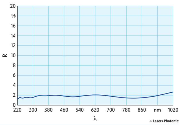
4 Super broadband anti-reflection coating for 220 up to 950 nm
