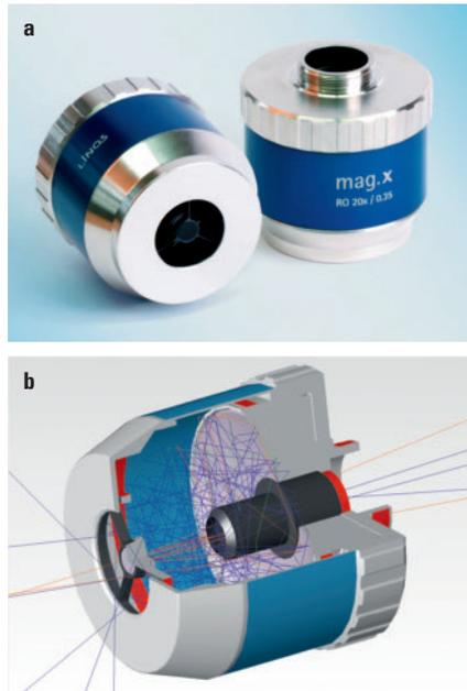
**3 UV-VIS mirror lens (a); evaluation of the stray light distribution in a mirror lens using non-sequential raytracing by TracePro software (b)**
