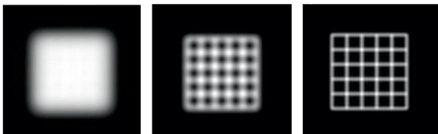
1 Simulation of the resolution increase by reducing the wavelength: Illustration of a test structure at (a) 1064 nm, (b) 532 nm and (c) 266 nm in an aberration-free optical system
